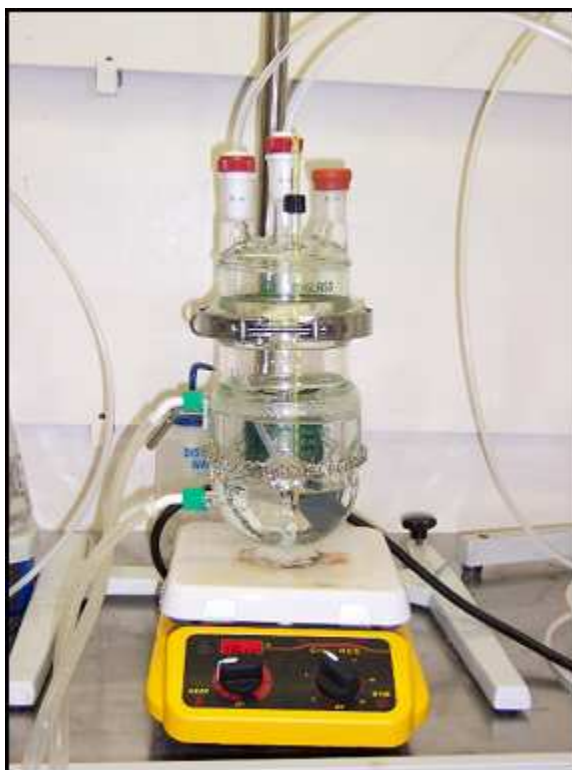
Figure 9.1: Reactor assembly for oleic acid ozonolysis at ambient pressure
