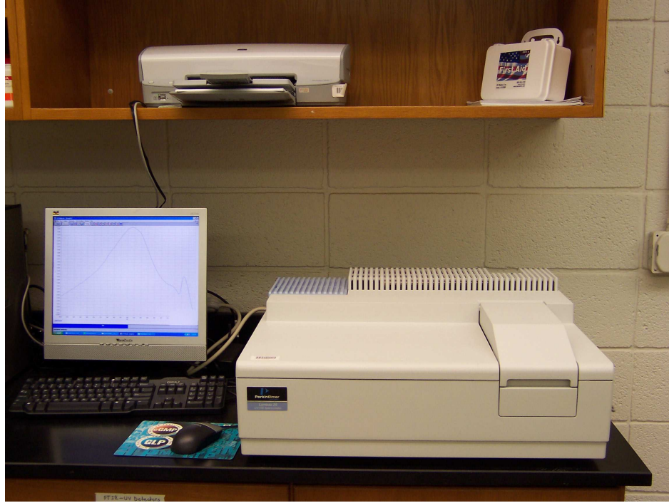
Figure 4.12: LAMBDA 25 UV/VIS Spectrophotometer used for determining potassium permanganate concentration
