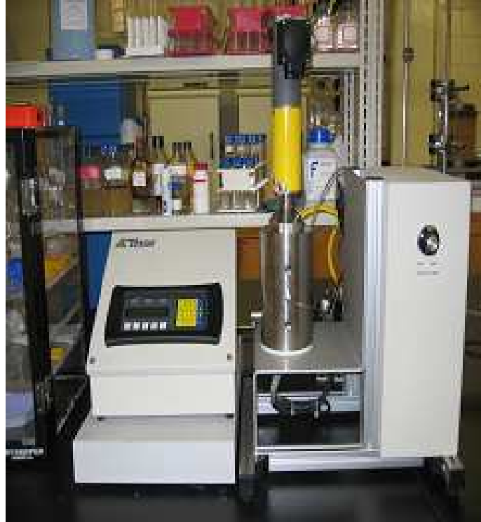
Figure 9.2: Reactor assembly for oleic acid ozonolysis in supercritical carbon dioxide
