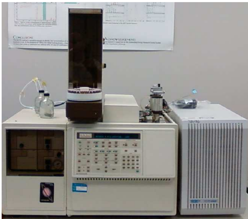
Figure 4.10: Varian 3600 GC with Saturn 2000 Mass Spectrometer used in this study
