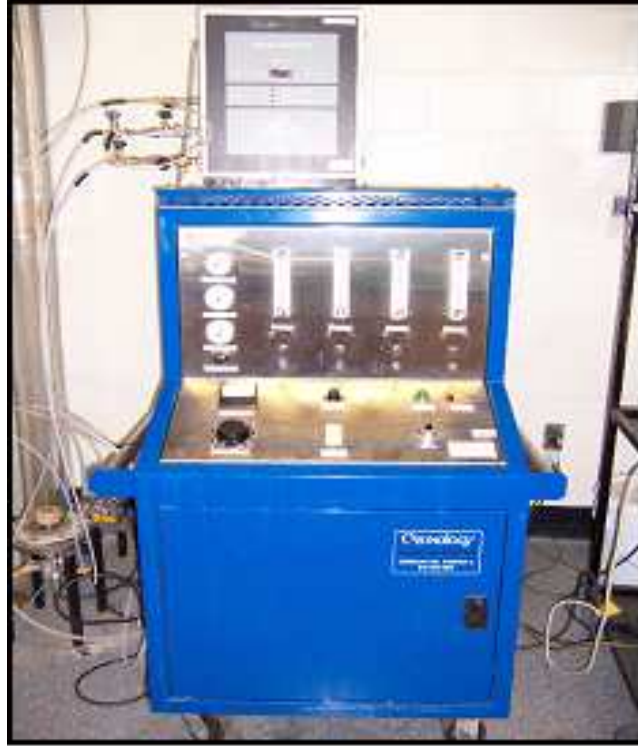
Figure 4.1: LC-1234 Ozone Generator equipped with a Model HC Ozone Monitor utilized for this study
